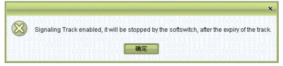
The system will monitor all signals arriving in the next 5 minutes. (The time can be specified in <System parameters>). All phone records created within this time period contain a full record of signaling process, which can be view by choosing <Signaling analysis> in the right-click menu.
